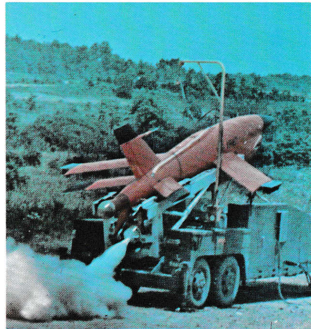
BQM—the most versatile target presented on the Range. The BQM can be launched from the air, from the ground, or at sea. After its 60-minute flight, the drone parachutes into the ocean. VC-8 helos bring the targets back to the Ryan Drone Repair Facility, where the BQM's are readied for another flight.
