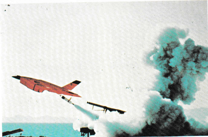
Firebee target drone being launched from a surface launch area.
